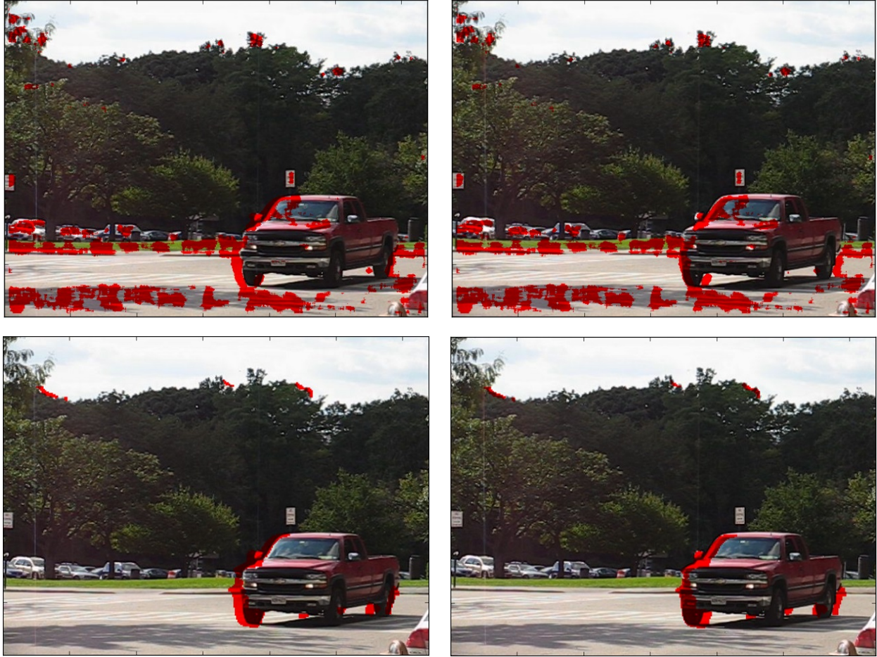
Figure 5.3: Oclusion detection between frames 7 and 8 of “Cars8” sequence of the Berkeley Motion Segmentation dataset. The occlusion (and disocclusion) areas are displayed on both frames. The image pair on top is obtained with the baseline algorithm, which gives many false alarms on turbulent and with variant lightning scene areas, such as the road and the car’s front surface. The image pair below displays our detection having used the aggregate superpixel distance from Eq. 5.9 and m = 8 superpixel maps.
