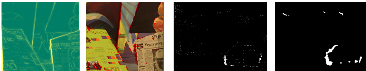
Figure 5.6: The left image pair compares our method with an algorithm that considers both flow and boundary features [74] on the hard, short-baseline “Venus” sequence from the Middlebury dataset. Our method (right) is able to disregard most edges which are not occlusion boundaries. However, although superpixels drive the occlusion boundaries, flow features still occasionally display better behavior on boundaries. In the right image pair we compare our algorithm with a state-of-the-art optical flow algorithm [11] on the “Cars8” sequence. Our method (right) is more accurate, especially on areas with varying illumination, such as the windscreen and the car shadow.
