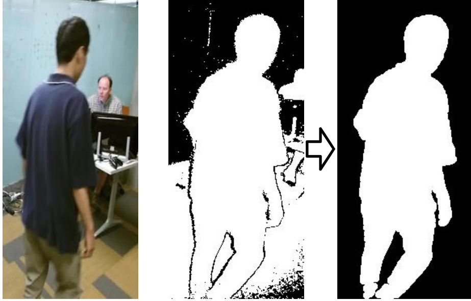
Figure 4.2: The cropped color image (left), the grayscale depth representation D_p^g (center) and the result after background subtraction (right) using the body index information B_p from skeleton tracking.
