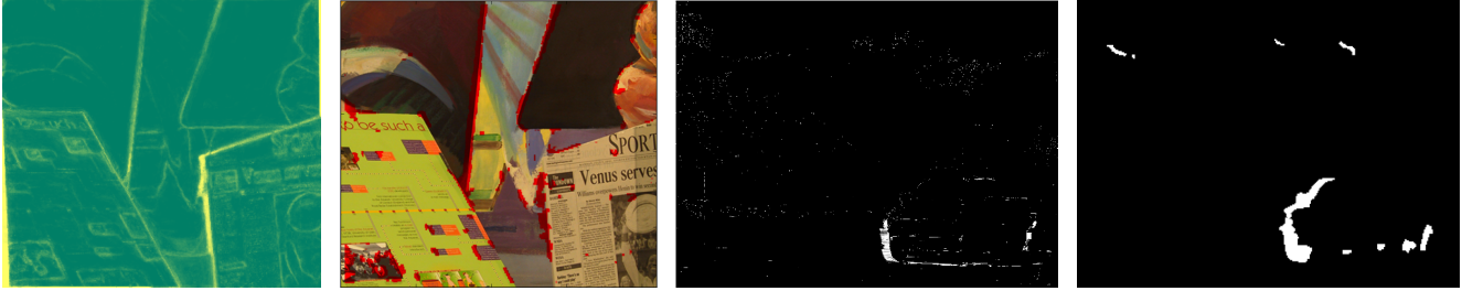
Figure 6: The left image pair compares our method with an algorithm that considers both flow and boundary features [14] on the tough, short-baseline “Venus” sequence from the Middlebury dataset. Our method (right) is able to disregard most edges which are not occlusion boundaries because of affine-invariance; they are visible on different positions of compared patch pairs that include them. However, although superpixels drive the occlusion boundaries, flow features still occasionally display better behavior on boundaries. In the right image pair we compare our algorithm with a state-of-the-art optical flow algorithm [3] on the “Cars8” sequence. Our method gives more accurate occlusion detection, especially on areas with varying illumination, such as the windscreen and the shadow of the car. This should be compared to the ground truth in Fig. 4.
