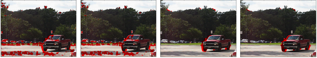
Figure 3: Occlusion Detection between frames 7 and 8 of the “Cars8” sequence of the Berkeley Motion Segmentation dataset. The occlusion (and disocclusion) areas are displayed on both frames. The left image pair is obtained with the baseline algorithm, which gives many false alarms on turbulent and with variant lighting scene areas, such as the road and the car’s front surface. The right image pair displays our detection having used the aggregate superpixel distance from Eq. 9 and m = 8 superpixel maps.
