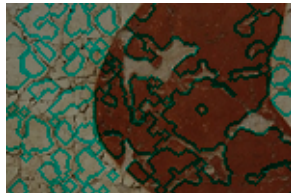
(b) Crack detection
